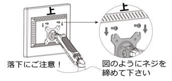
(3) Install the lower two screws and fasten the upper two screws.
